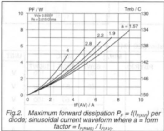
Fig.2. Maximum forward dissipation  $P_F = f(IF_{AV})$  per diode; sinusoidal current waveform where  $a = \text{form factor} = I_{F(RMS)} / I_{F(AV)}$ .
