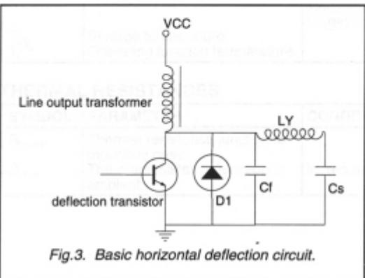
Fig. 3. Basic horizontal deflection circuit.
