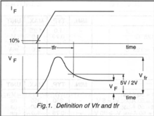
Fig. 1. Definition of  $V_{fr}$  and  $t_{fr}$
