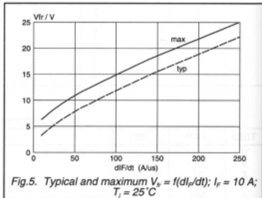
Fig. 5. Typical and maximum  $V_{fr} = f(dI_F/dt)$ ;  $I_F = 10 \text{ A}$ ;
