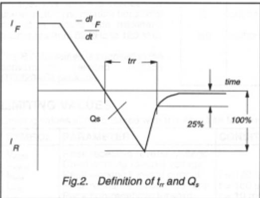
Fig. 2. Definition of  $t_{rr}$  and  $Q_s$
