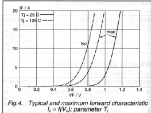
Fig. 4. Typical and maximum forward characteristic
